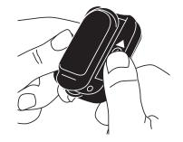
3. Slide the battery door away from you and off the device.
