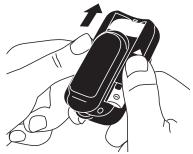
4. If applicable, remove the old batteries. Properly dispose of the batteries.
