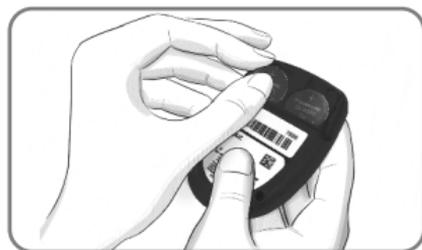
4. Make sure the '+' sign is facing up on the new batteries.
