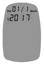
Once you insert the batteries the device will automatically enter the set-up mode. The YEAR will be flashing on the LCD Screen.
