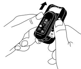
4. If applicable, remove the old batteries from the 3240. Properly dispose of the batteries.
