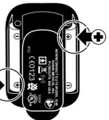
6. Carefully slide the battery door back onto the device.
